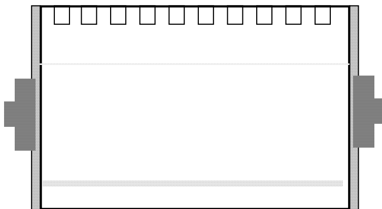
Gel as it is likely to appear near end of run-- Fuzzy line near bottom is tracking dye; proteins are not yet visible.
