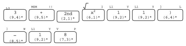
We now wish to change the second 1 in 11 to a 0. Press the left arrow key, located on the right side in the 2nd and 3rd rows, 5 times. The blinking cursor should be above the 1. Press the 0 key followed by the ENTER key. The result, -11.83772234, should be displayed. (NOTE: If you calculator is not set to the "Float" mode, you may display fewer digits in the result.)
