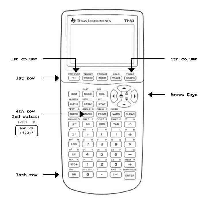
ON/OFF - Most of the calculator keys serve more than one purpose. The ON/OFF key, located in the 10th row and 1st column of the calculator, is used to both turn the calculator on and to turn the calculator off. Notice that "OFF" appears in gold print. This indicates that this is a 2nd function of the key and is accessed by first pressing the "2nd" key, located on the 2nd row, 1st column.
