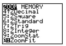
Observe ZoomFit in the O position. Since your cursor is at this position, you can press ENTER to activate ZOOM FIT or you could have pressed the O key without using the DOWN ARROW. Press ENTER or O now.
