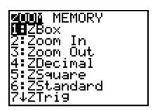
Your calculator display should appear as the screen above. ZOOM STANDARD is on the 6th line and may be activated by moving the cursor down to "6:ZStandard" with the arrow keys then pressing ENTER or by simply pressing the 6 key.
