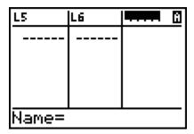
Type ABC then (ENTER). It is not necessary to press the ALPHA key.
