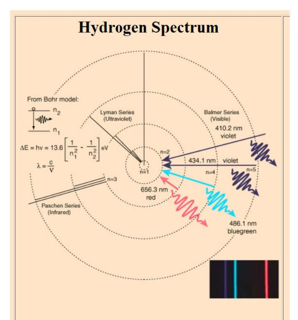
This spectrum was produced by exciting a glass tube of hydrogen gas with about 5000 volts from a transformer. It was viewed through a <u>diffraction</u> grating with 600 lines/mm. The colors cannot be expected to be accurate because of differences in display devices.
