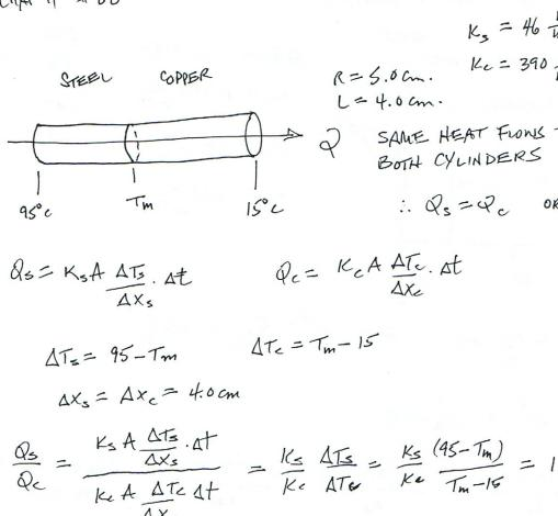
$$\frac{Q_{S}}{Q_{C}} = \frac{K_{S} A \frac{\Delta T_{S}}{\Delta X_{S}} A + \frac{\Delta T_{S}}{\Delta X_{S}} A + \frac{K_{S}}{\Delta X_{S}}}{K_{C} A + \frac{\Delta T_{C}}{\Delta X_{C}} A + \frac{K_{S}}{\Delta X_{C}}} = \frac{K_{S}}{K_{C}}$$
