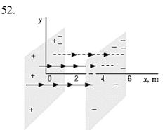
An infinite plane of surface charge density  $\sigma = +8.00 \text{ nC/m}^2$  lies in the yz plane at the origin, and a second infinite plane of surface charge density  $\sigma = -8.00 \text{ nC/m}^2$  lies in a plane parallel to the yz plane at x =4.00 m. The electric field at x = 5.00 m is approximately A) 226 N/C B) 339 N/C C) 904 N/C D) 452 N/C E) zero
