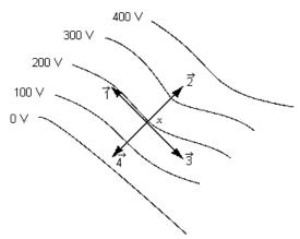
The vector that best represents the direction of the electric field intensity at point x on the 200-V equipotential line is
