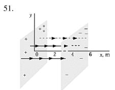
An infinite plane of surface charge density  $\sigma = +8.00 \text{ nC/m}^2$  lies in the yz plane at the origin, and a second infinite plane of surface charge density  $\sigma = -8.00 \text{ nC/m}^2$  lies in a plane parallel to the yz plane at x = 4.00 m. The electric field at x = 3.50 m is approximately
