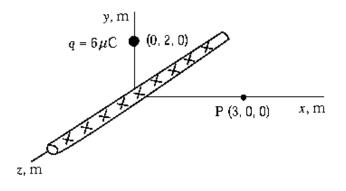
An infinite line charge of linear density λ = 0.30 µC/m lies along the *z* axis and a point charge *q* = 6.0 µC lies on the *y* axis at *y* = 2.0 m. The *x* component of the electric field at the point P on the *x* axis at *x* = 3.0 m is approximately
