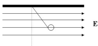
A bob of mass m (m = 0.500 g), and charge magnitude Q ( $Q = 50.0 \mu$ C) is held by a massless string in a uniform electric field E. If the bob makes an angle of 10.0 degrees with the vertical, then calculate the magnitude of the electric field E and the sign of the bob charge Q.
