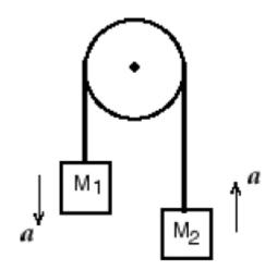
The basic intent of the Atwood Machine is to slow down the motion so that the system acceleration is easier to measure. Then, by applying Newton's 2<sup>nd</sup> Law to the system, the above equation for the calculated acceleration can be derived, where friction has been explicitly ignored.
