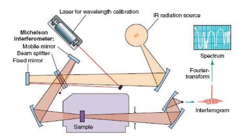
\* The position of an absorption band (peak) in an IR spectrum is specified in units of wavenumbers ( $\overline{v}$ )
