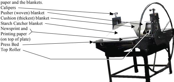
**Remember:** To **loosen** the top (pressure) roller turn the calipers counter-clockwise
