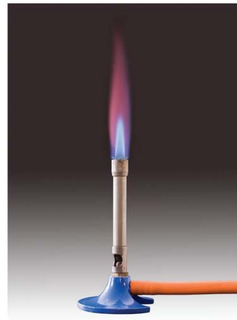
**Bunsen Burner** A laboratory burner that uses natural gas for fuel.
